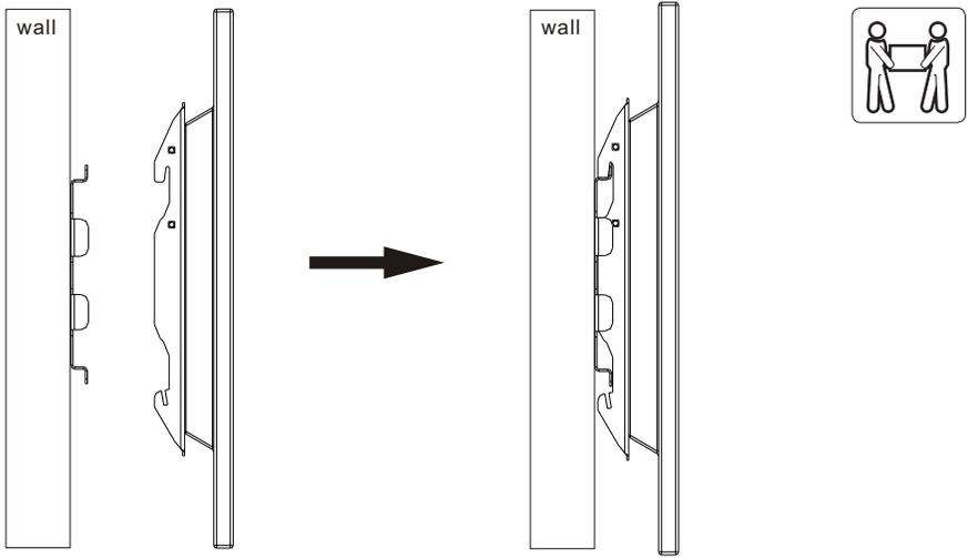
Lift your TV and hook the top hooks over the top of wall plate rail.
