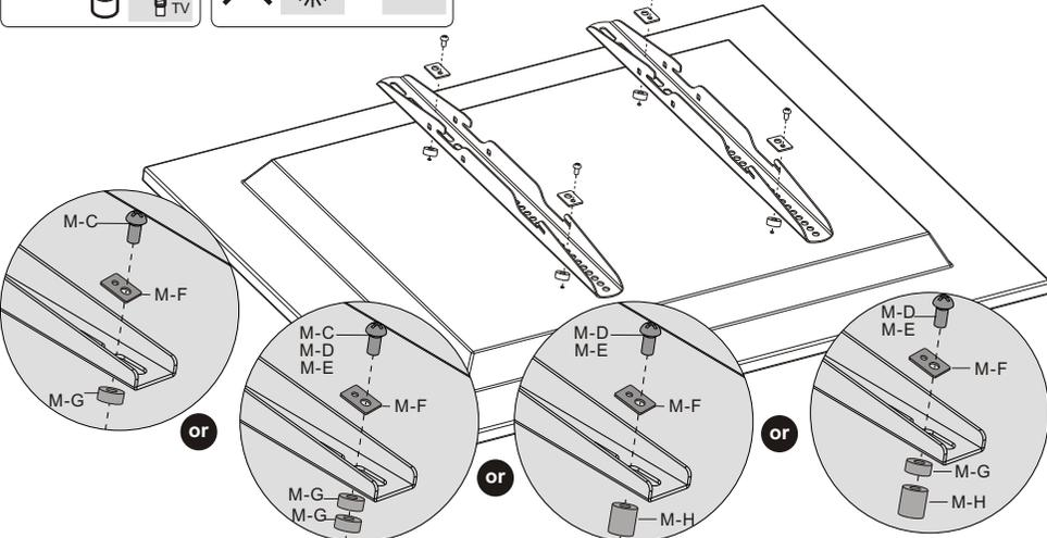
**Note:** Choose the appropriate screws, washers and spacers (if necessary) according to the type of screen.
