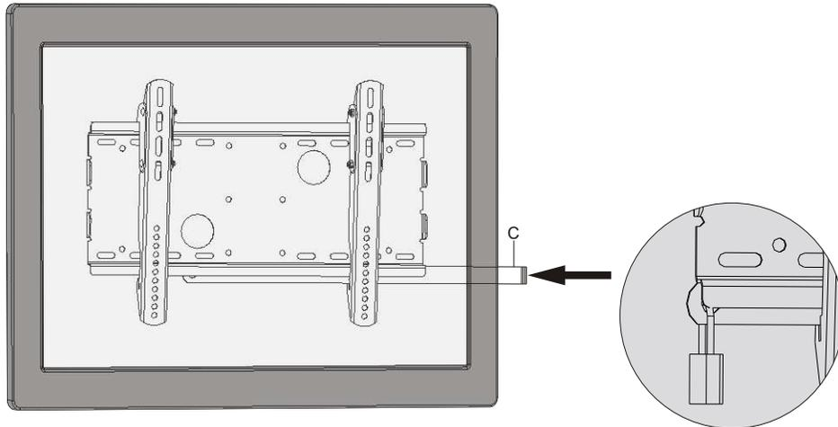
Insert the safety bar to secure the rails.
