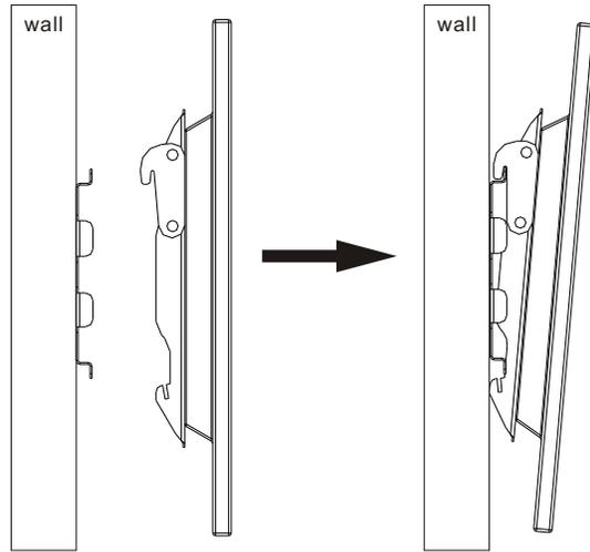
Attach the tilt options to the TV rails using supplied screws and lock nuts.
