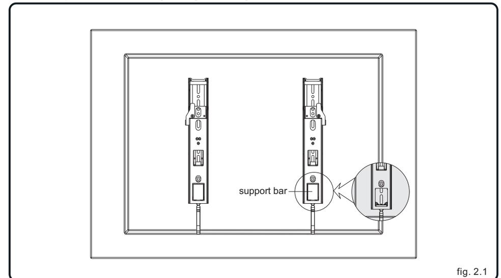
**NOTE:** For flat back screens proceed to step 2-1. For bump-out or recessed back screen skip to step 2-2.
