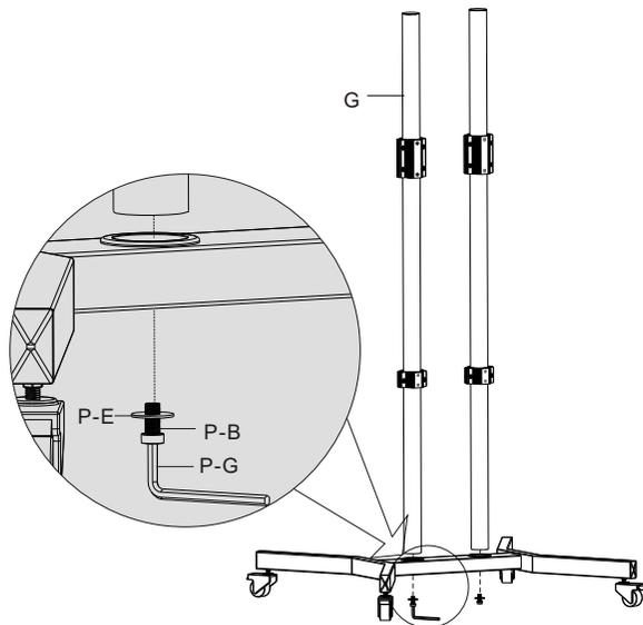
Attach two pillars to base using screws and washers, tighten screws using 8mm Allen key.
