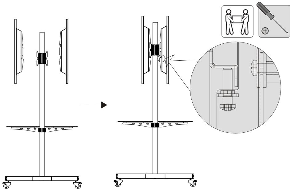
Tighten the bottom bolts to secure the adapter brackets to the universal plates.
