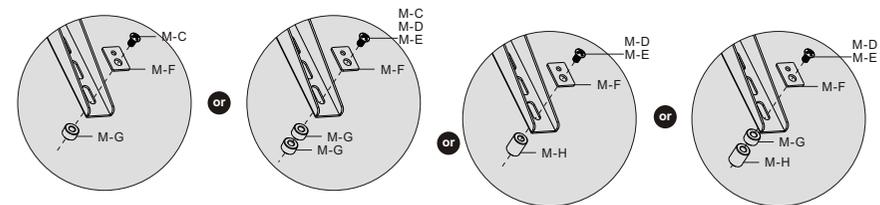
**Note:** Choose the appropriate screws, washers and spacers (if necessary) according to the type of screen.
