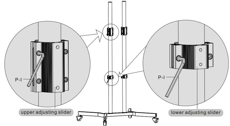
Loosen the screws on upper adjusting slider and adjust them to desired position using 5mm Allen key. Adjust the height of the lower adjusting sliders to desired position in the same way.
