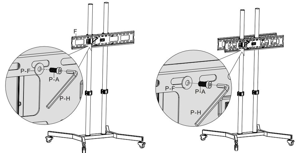
Fix the universal plate on the upper adjusting sliders, using the appropriate combination of screws and washers, make sure the universal plate is level, tighten all screws using 6mm Allen key. Do the same step as above for the other universal plate.
