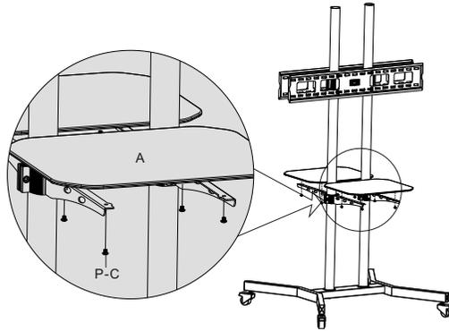
Place glass shelf on supporting arm, using the appropriate screws to fix the shelf, do not over tighten, otherwise may cause glass to shatter or crack. Do the same step as above for the other glass shelf.
