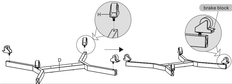
Insert four wheel casters into holes of base and tighten the nuts of wheel casters to secure.
