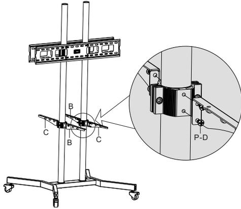
Fix the supporting arm to the lower adjusting slider, using the appropriate combination of screws, make sure the supporting arms are level, tighten all screws.
