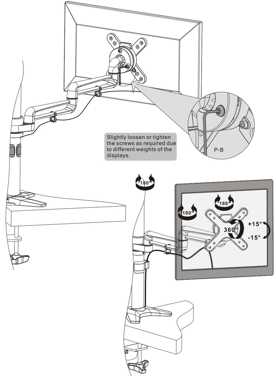
Slightly loosen or tighten the screws as required due to different weights of the displays.
