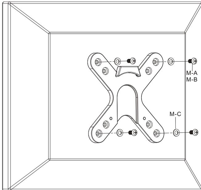
Screw the VESA plate onto the display.
