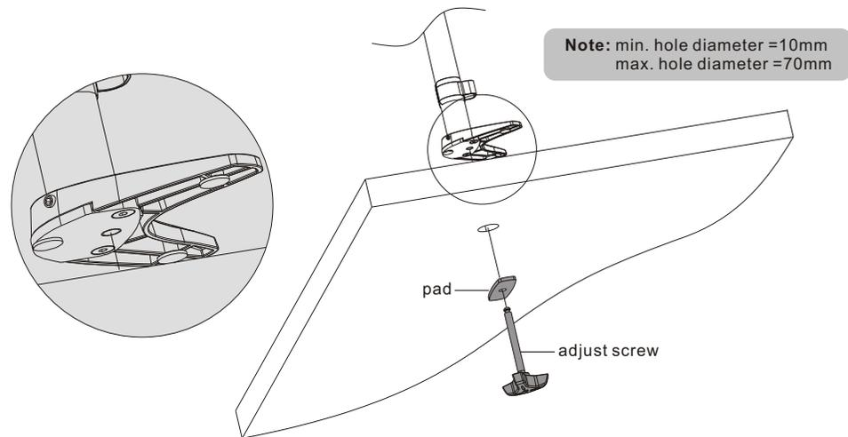
Insert the adjust screw into base plate through the hole. Then using the adjust screw to fix and tighten it securely.
