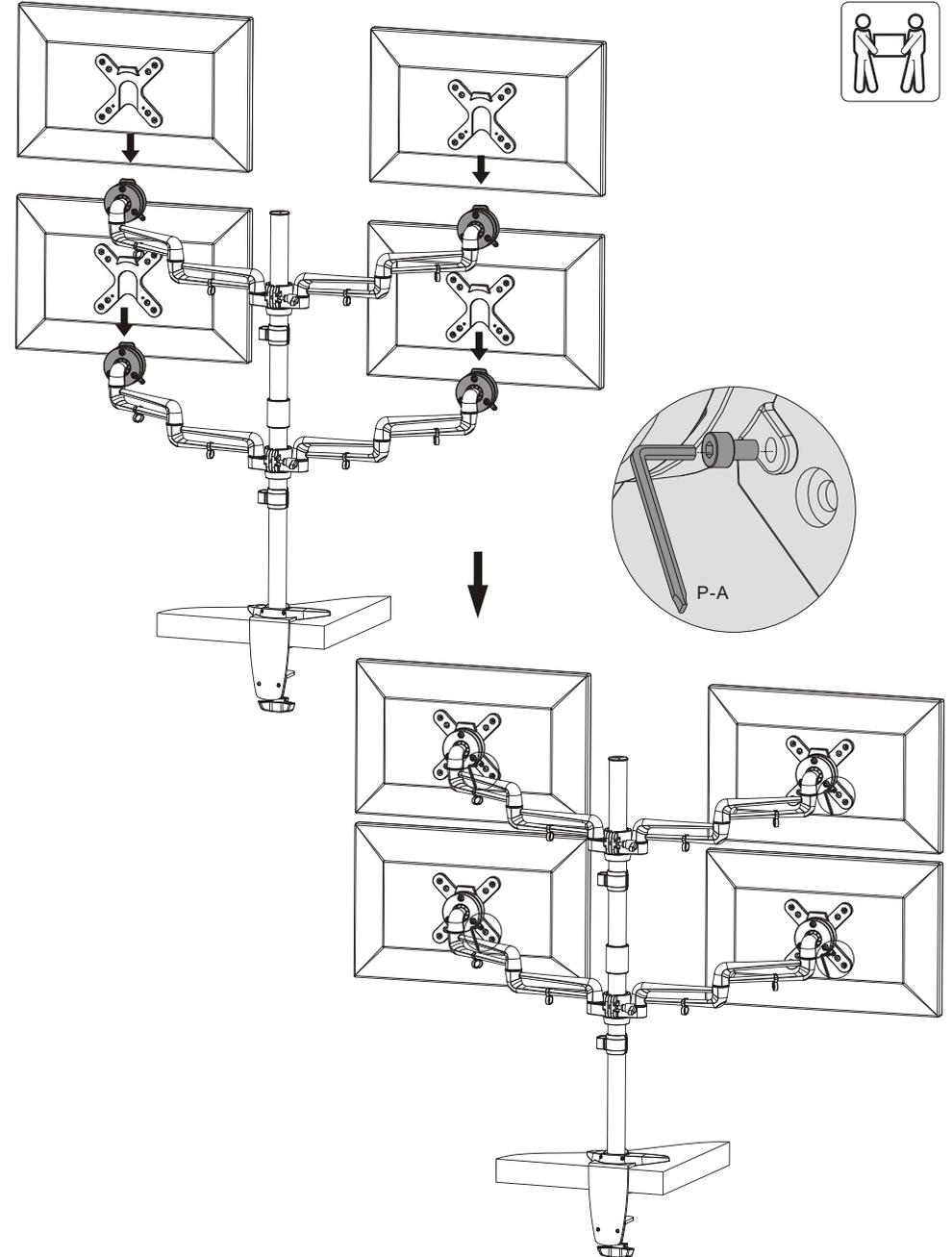
Insert the VESA plate onto the mount and use the previously removed screws to secure them. Make sure the display is safely secured before finally releasing.
