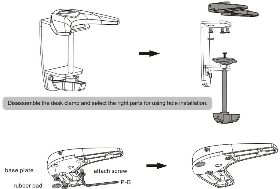
Re-install the base plate with three retained screws, then tighten securely.
