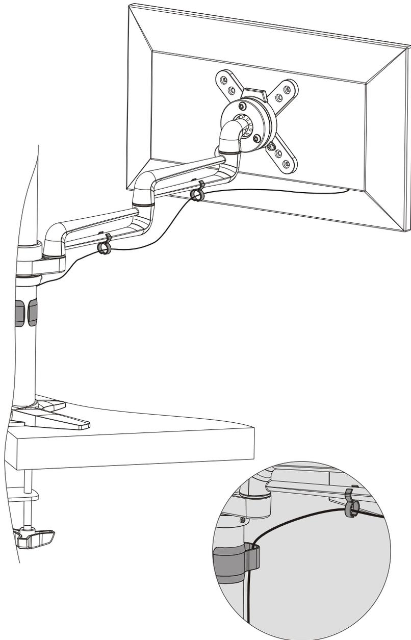
Use clips for routing the cables.
